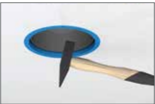
Knock in ventilation sleeve from below with hammer.
