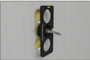
Open quick-release lever and insert in existing hole.
