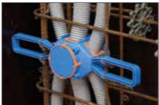
Standard spacing to door frame 15 cm. Suitable for up to 6 installation pipes M20/25 or 4x M20/25 plus 2x M32 - also rigid pipes.
