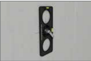
The drill template is attached by closing the lever.
