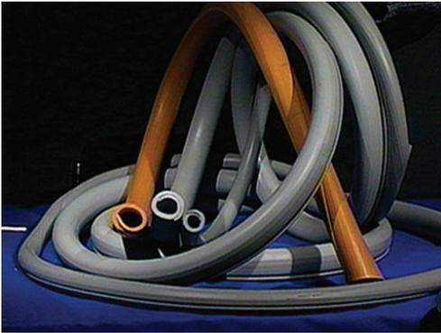
E/Insulation is a silicone hose used to protect a variety of distribution and substation equipment up to 20 kV phase-to-ground. The E/Insulation is manufactured with a split seam to allow for an easy application without the need of breaking electrical connections. The hose is simply pulled and split apart allowing it to be quickly slipped over the cable or bus being protected. There is no heat shrinking required for application and no tools other than a cutting tool for proper length are needed.
