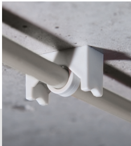
With the FS Fixing mounting base in connection with the DKS Dowel clamp, the effortless mounting of thermal conduction cables with a fixed distance of 8 or 15 mm to the ceiling is possible.
